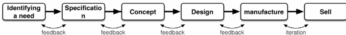
Figure 7: Conclusion of design process models adopted and interpreted from the source: (Roy, 2006:25)
